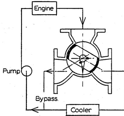
Fluid temperature below operating range — no flow to cooler
