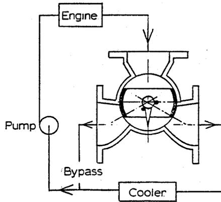
Fluid temperature in operating range — flow proportioned between bypass and cooler
