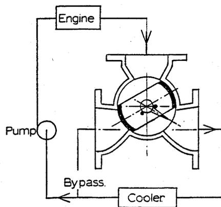
External lever in 'full flow to cooler' position.
